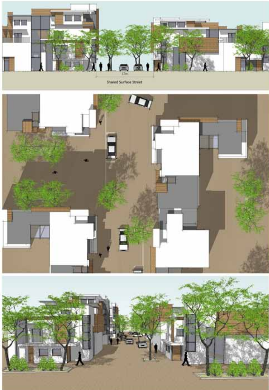
Figure 15.11 Shared Surface Street
