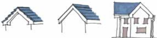
Figure 16.29 Avoid roofs with large overhangs which result in the roof sitting like a 'lid' on the building.
