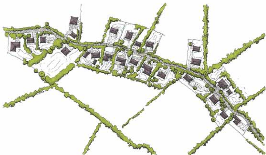
Figure 16.1 Houses positioned parallel to the public road in the form of ribbon development and irrespective of site analysis and desirable orientation which leads to a loss of the rural character of the area.
