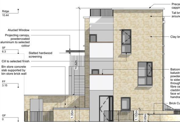
02A 1B/2P Triplex - Elevation A
