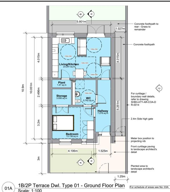
01A 1B/2P Terrace Dw. Type 01 - Ground Floor Plan
