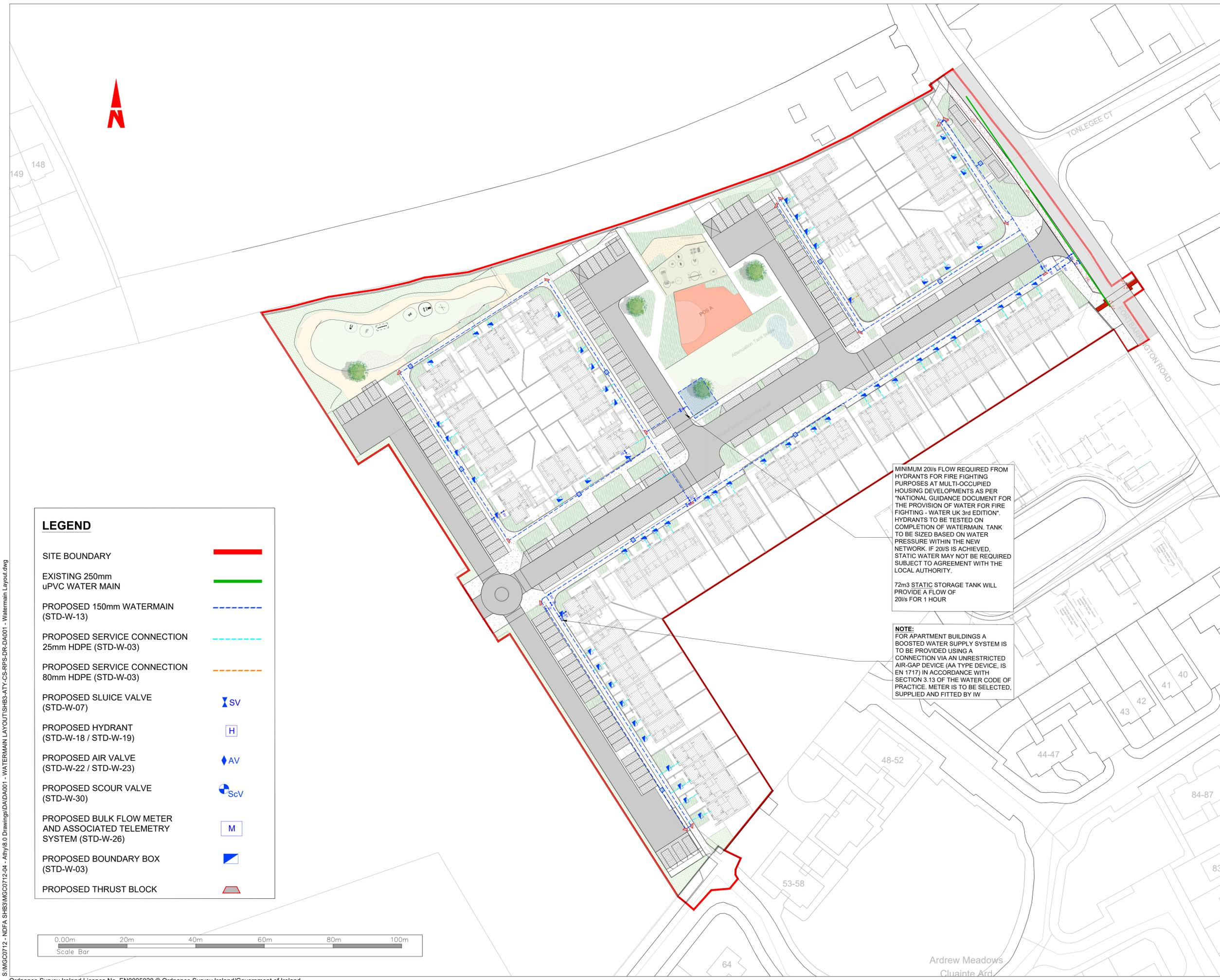
MINIMUM 20l/s FLOW REQUIRED FROM HYDRANTS FOR FIRE FIGHTING PURPOSES AT MULTI-OCCUPIED HOUSING DEVELOPMENTS AS PER "NATIONAL GUIDANCE DOCUMENT FOR THE PROVISION OF WATER FOR FIRE FIGHTING - WATER UK 3rd EDITION". HYDRANTS TO BE TESTED ON COMPLETION OF WATERMAIN. TANK TO BE SIZED BASED ON WATER PRESSURE WITHIN THE NEW NETWORK. IF 20l/s IS ACHIEVED, STATIC WATER MAY NOT BE REQUIRED SUBJECT TO AGREEMENT WITH THE LOCAL AUTHORITY.
