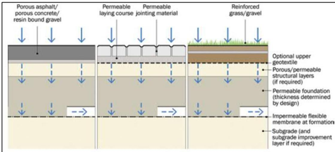
Figure 9: Porous Surfacing System - No Infiltration (Source: CIRIA C753 SuDS Manual)
