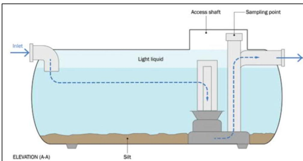
Figure 12: Typical Petrol Interceptor Detail (Source: CIRIA C753 SuDS Manual)
