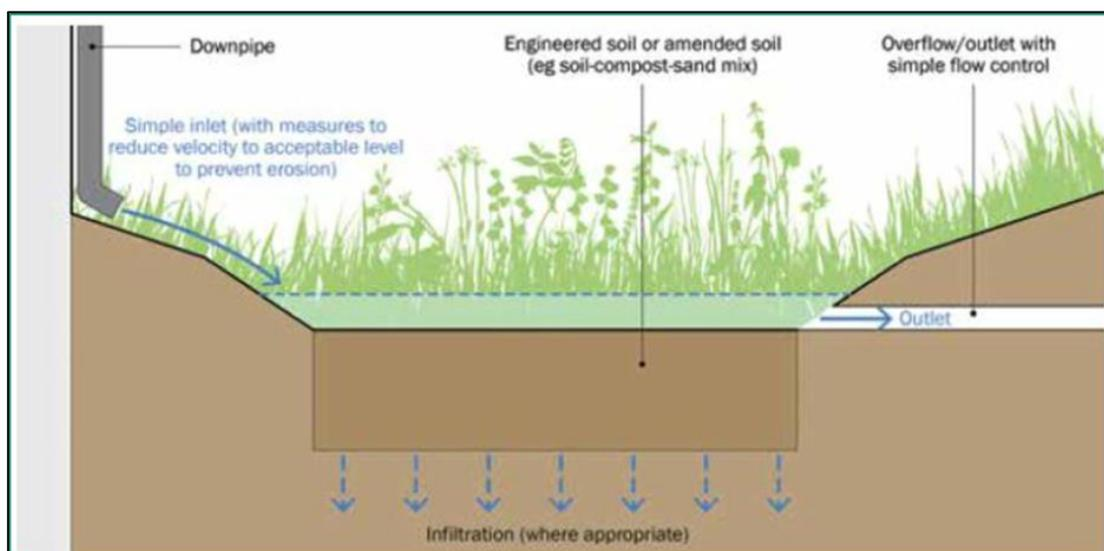
Figure 10: Typical Bio-Retention Section (Source: CIRIA C753 SuDS Manual)
