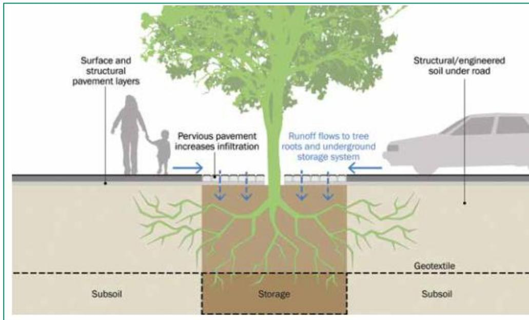
Figure 11: Collection of Surface Water Runoff for Trees (Source: CIRIA C753 SuDS Manual)
