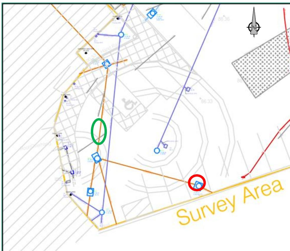
**Figure 13: Existing Foul Pipes to be Amended as part of the Works**
