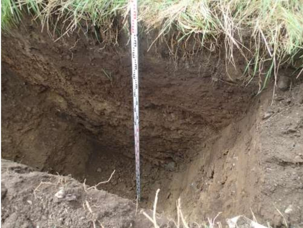
**Plate 3: Profile of soil and subsoil in trial hole number 2. See the well aerated nature of the topsoil and the subsoil, with no mottling throughout the profile. See again the absence of bedrock and the water table at 3.1m below ground level.**
