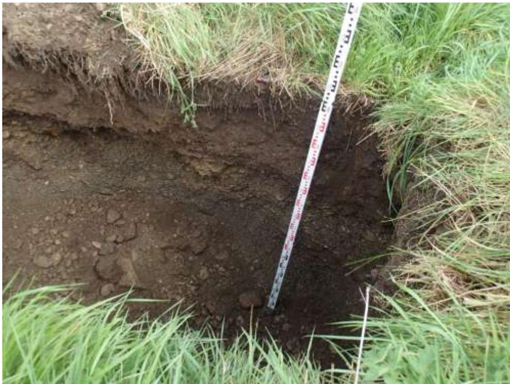
**Plate 2: Profile of soil and subsoil in trial hole number 1. See the well aerated nature of the topsoil and the subsoil, with no mottling throughout the profile. See also the absence of bedrock and the water table at 2.1m below ground level.**
