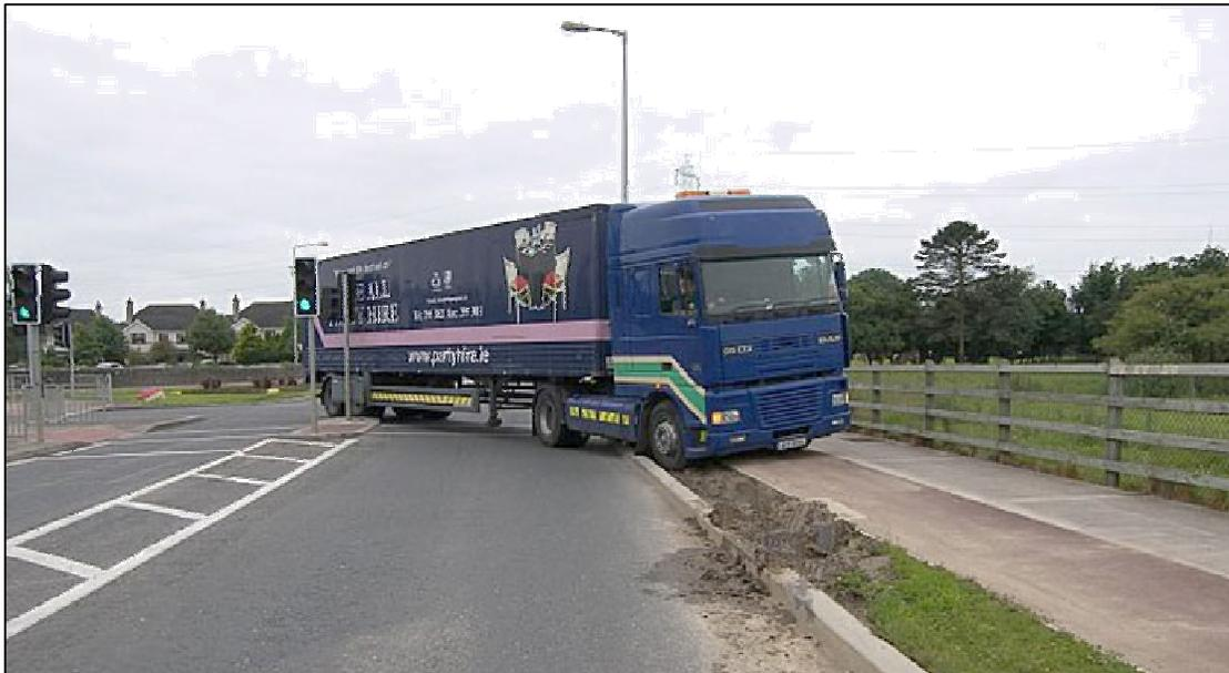
**Plate 8: Over-running at the Clane Road/Shackleton Road junction, Celbridge**
