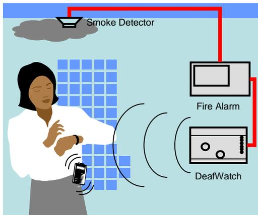
The diagram on the left demonstrates the basic operational principles of DeafWatch.
