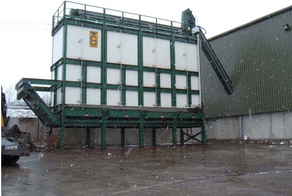
Figure 4.4: Greenstar – Vertical Composting Unit (VCU) at Silliot Hill
