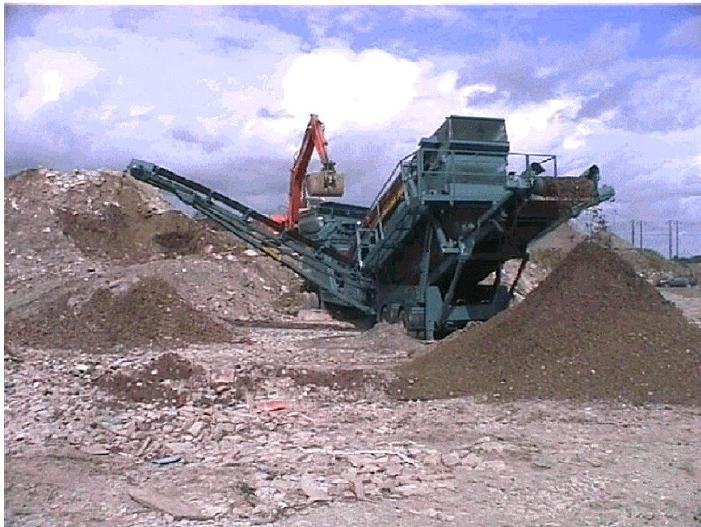
Figure 6.5: Recycling of Construction & Demolition Waste at Kinsale Road Sanitary Landfill
