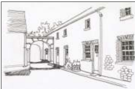
Figures 23 & 24: Images of the type of architectural form around which new developments should be based, which takes its design form from the Georgian canal frontage. These design traits include vertical emphasis to windows, tall, steeply pitched roofs, some articulation of the front door, natural materials and finishes.
