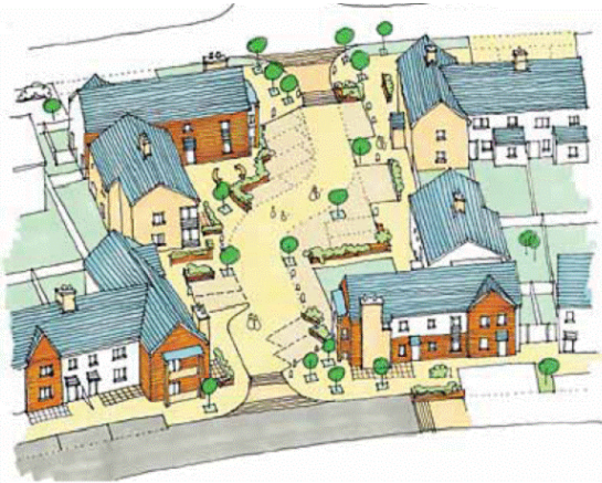
Figure 25: Layout to control traffic speed (Urban Design Manual 08).
